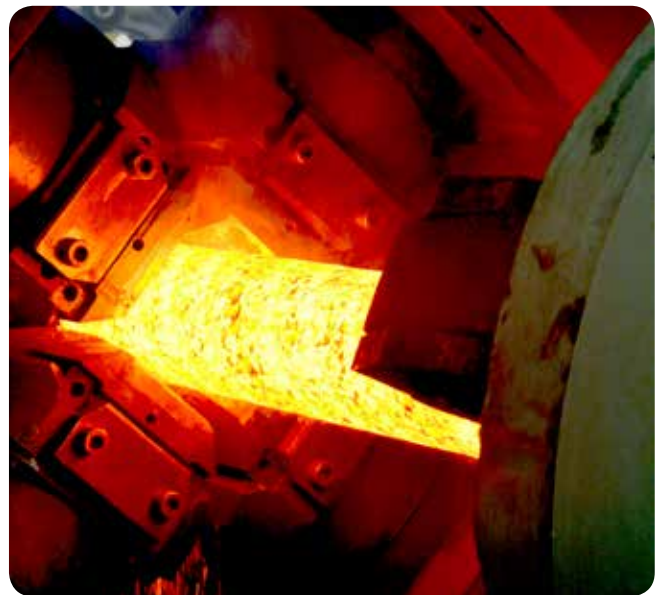
An M284 155 mm howitzer tube is forged at Watervliet Arsenal after it was heated in a state-of-the-art furnace installed through a public-private partnership with Electralloy. The tube was heated to nearly 2,000 degrees before the rotary forge pounded it into the near shape of a howitzer tube. (U.S. Army photo)
